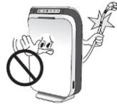
Stop using the device and call our A/S center when electric cord or plug is damaged.
