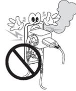
Do fully insert and fit electric plug into electric sockets.
